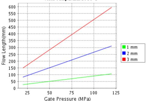
Note: Technical support is recommended if Gate Pressure is greater than 80 MPa. Contact your local representative. Moldflow is a registered trademark of the Moldflow
